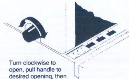
Turn clockwise to open, pull handle to desired opening, then turn knob counter-clockwise to lock.
