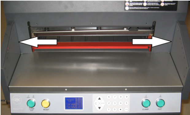
Figure 3. Infrared Safety Walls
