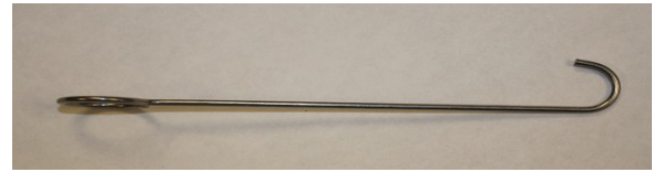
Figure 19. Cut Stick Removal Tool
