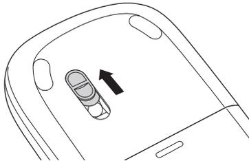
**IMPORTANT:** Placing the dongle into the mouse does NOT switch off the mouse. Taking it out does not switch it on either. The mouse is switched on or off ONLY by sliding the lens cover.
