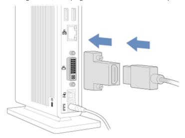
Note: If a DVI-to-HDMI adapter is not included with your Docking Station, you must purchase one separately to use the HDMI output. The HDMI output supports the video signal only. For the audio signal, you must use an adapter cable (sold separately) to connect the front or rear stereo audio output to external speakers or to the audio input on your monitor or TV.
