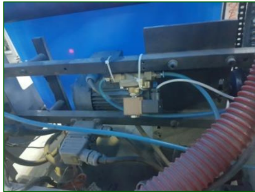
Use of solenoid valves decreases the need for pressurized air
